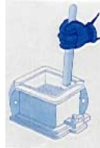
There are a number of items that must be stated in a report on the test to comply with the British or European Standard (**BS 1881 part 108 or BS EN 12390-2**), including where and when the cubes were made, size, cube ID and the name of the person making the cube. Other information is optional, such as the supplier, grade and workability and where the concrete was used in the structure.
